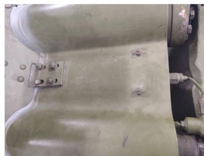
Fig. 3. Casing mounting on the recoil device casing of the D20 gun
