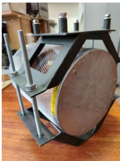
Fig. 6. Bracket for mounting RMPMD with SAP on self-propelled guns 2S1, 2S3
