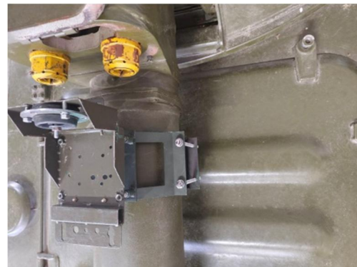
Fig. 7. Alignment of brackets for self-propelled guns 2S1, 2S3 with a bracket for a towed gun D20
